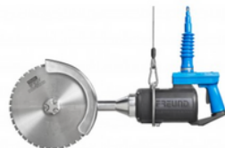
K32-06L CIRCULAR QUARTERING SAW
